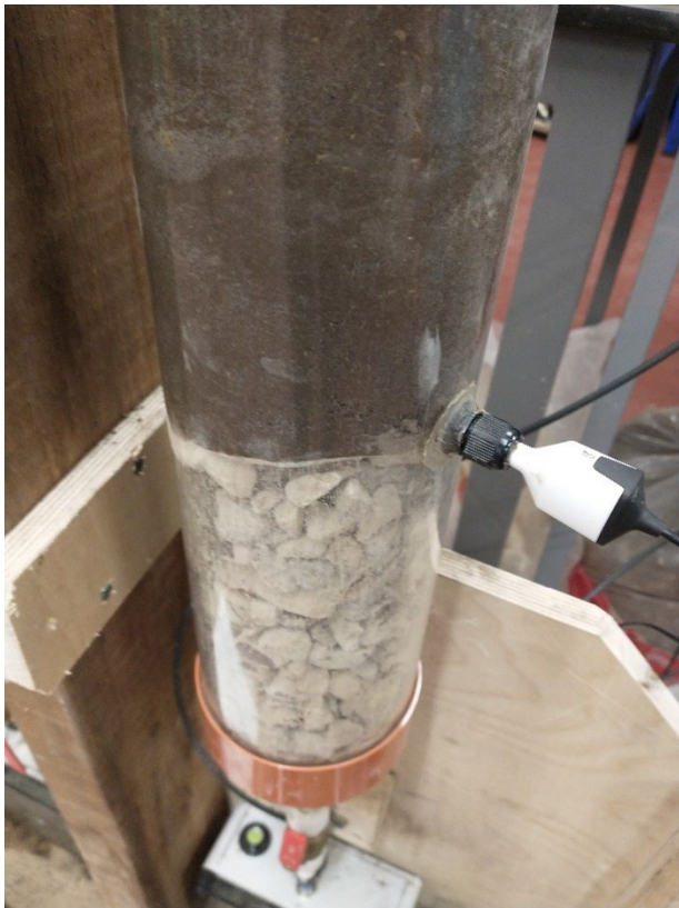
Fig. 4. Example of a column experiment showing the boundary between the coarse- and fine-grained materials.
