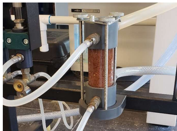
Fig. 7. Constant head permeability test
