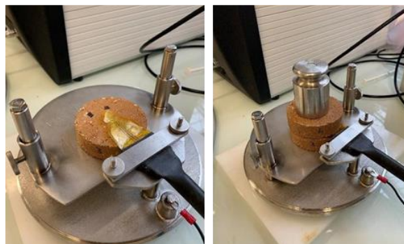
Fig. 2. Preparation steps for the Hot Disk measurement.
