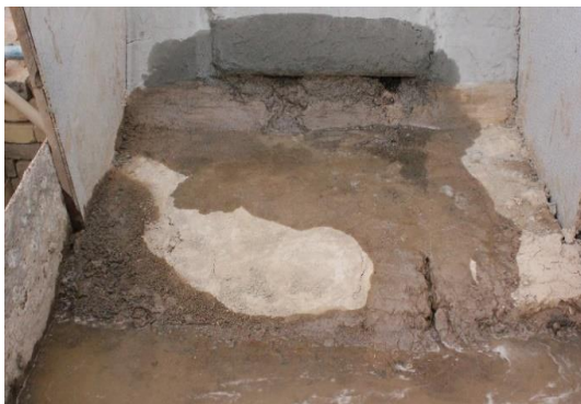
Fig. 3. Model of opening of the aquifer and groundwater outlet to the surface by gravity, the process of water outflow to the surface with the formation of primary deformations.
