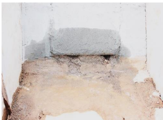
Fig. 4. The model of the opening of the aquifer and the release of groundwater to the surface by gravity, the end of the outflow of water, the frosting in the aquifer of the washout.
