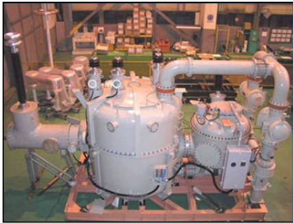
Fig. 12. 63 MVA/220 kV SF6 power transformer, produced by Russian Federation manufacturer.
