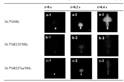
Changing the volume ratio of flame retardants/NH<sub>3</sub>, the flammability limits of R125/NH<sub>3</sub> and the flammability limits of R125/NH<sub>3</sub> and R227ea/NH<sub>3</sub> decreased gradually with the increase of the volume ratio and finally reached the critical flammability point. With reference to the existing studies, the GWP values and flammability limit ranges of binary mixtures can be calculated from the following two equations:
