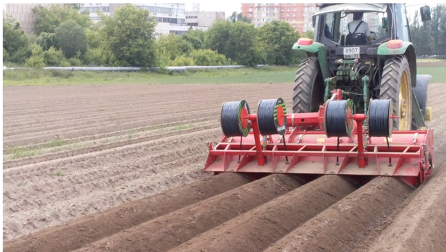
Fig. 3. Drip Tape Installer Based on Ridge Shaper Grimme GF-75/4.
