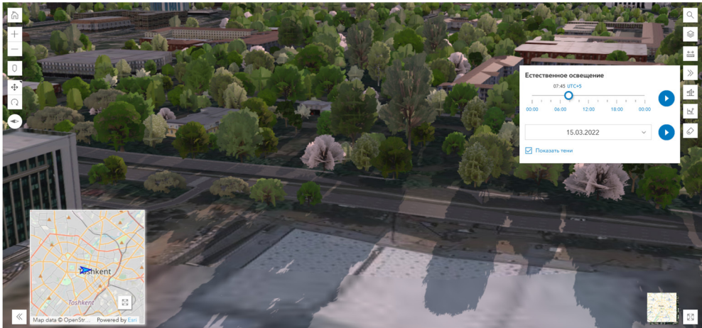
Fig. 10. With the Daylight Tool, the user will be able to adjust the effect of sunlight and shadows, including time, date, animation methods, and shadow display.
