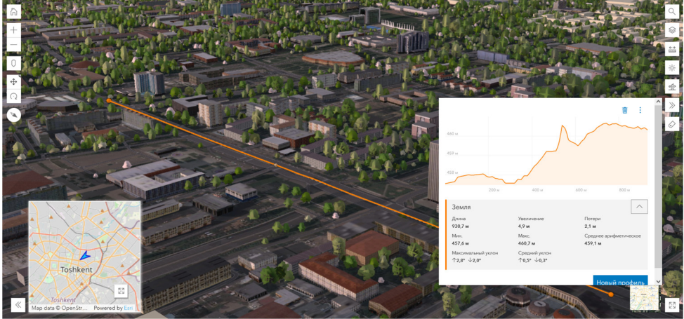
Fig. 9. Tool for creating a relief profile, where it is quite simple for the user to draw a line to obtain information about the relief profile of the selected direction.
