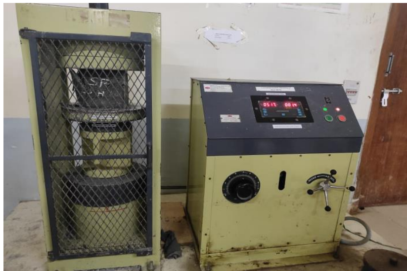
Fig. 3. Compressive strength test on steel fibre in bacterial concrete
