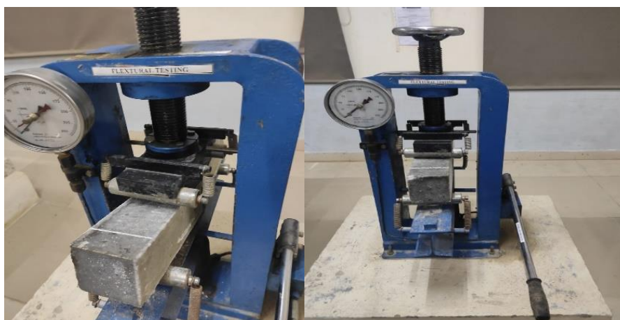
Fig. 7. Flexural strength test on steel fibre in bacterial concrete
