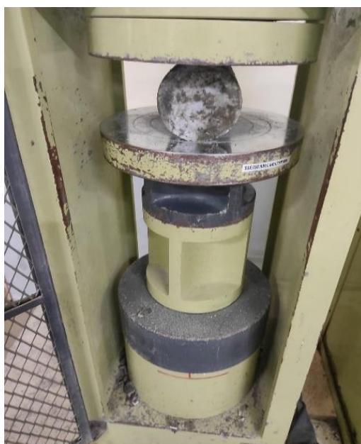
Fig. 5. Split tensile strength test on steel fibre in bacterial concrete
