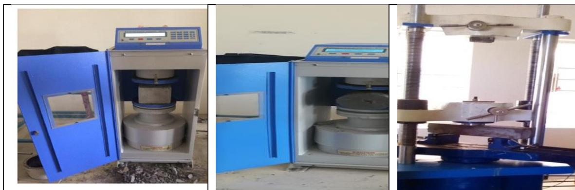
Fig 14 (a) Compressive strength (b) Split Tensile strength (c) Flexural Strength
