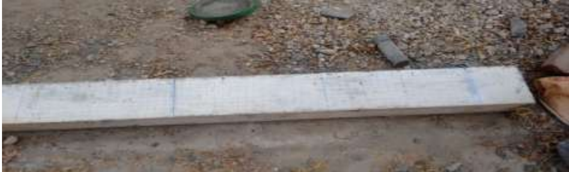
Figure 3.5 Cast specimen for cyclic loading
