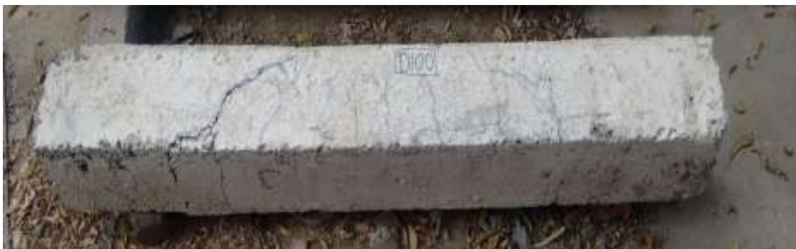
Figure 4.13 D100 beam after cyclic loading
