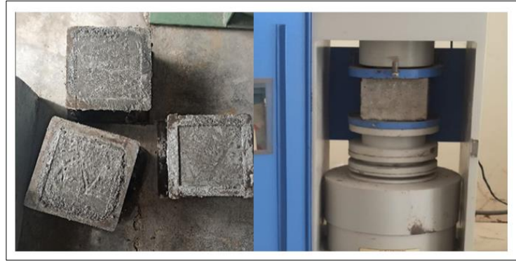
Fig 3: Cube specimen for ARGFRC-layer 1.
