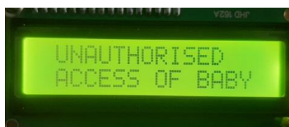
Fig. 16 LCD displaying the denial of authority
