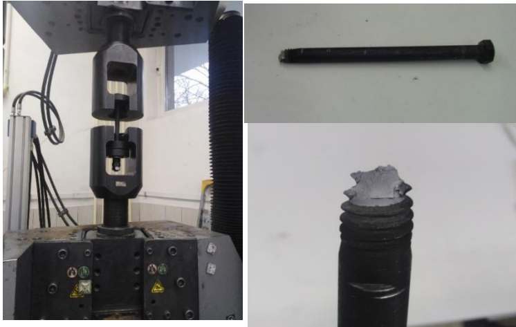
Fig. 1. Left: Installation of a high-strength bolt in a testing machine. Right: bolt failure along the threaded portion of the bolt.
