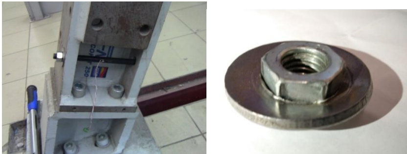
Fig. 2. Left: Testing the bolt on the stand. Right: piercing of the washer.
