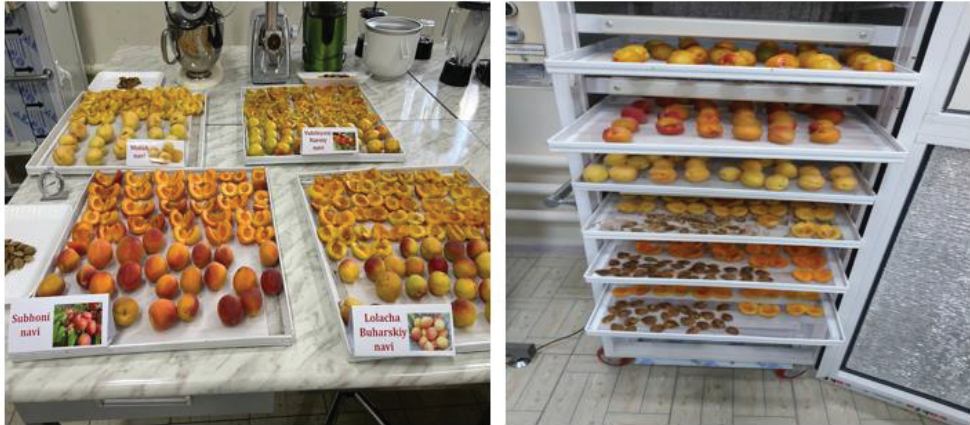
Fig. 2. The process of drying apricots taken for research in artificial drying equipment in laboratory conditions.
