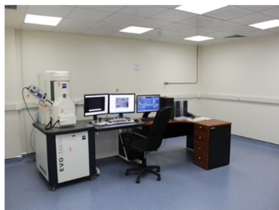
Fig. 2. SEM EVO MA (10) Zeiss scanning electron microscope. 1 – test bench with automatic high/low vacuum system and electronic control systems; 2 – chambers for samples; 3 – electron-optical system (handle); 4 – x-ray energy dispersive X-ray spectrometer (Oxford Instrument NanoAnalysis); 5 – secondary electronic detector (SE), 6 – monitor (3 pcs), 7 – keyboard and joystick; control computers (3 pcs); 8 – electronic blocks of the X-ray spectrometer; 9 – processors (3 pcs).
