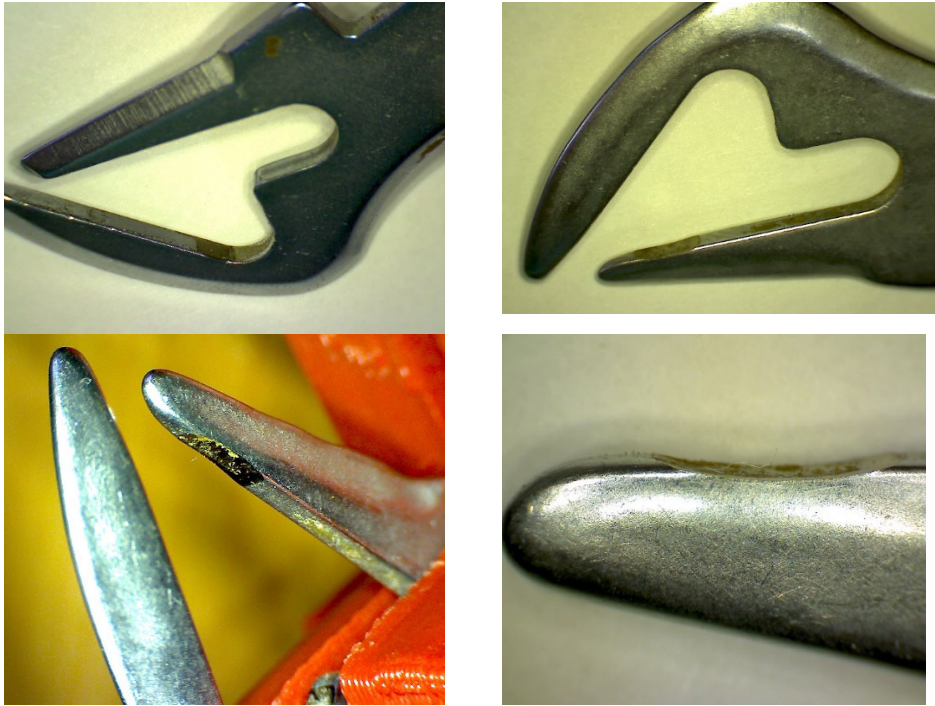
Fig. 1. Wear of the inner contact surfaces of the batten teeth.
