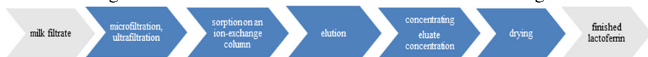
Fig. 1. Block diagram of LFh extraction from milk filtrate on the pilot equipment.
