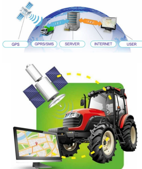
Fig. 2. Typical GPS monitoring system.
