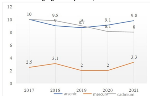
Fig. 5. The indicators of the content of arsenic, mercury and cadmium in the sewage sludge of 'Orelvodokanal', mg/kg of a dry basis.
