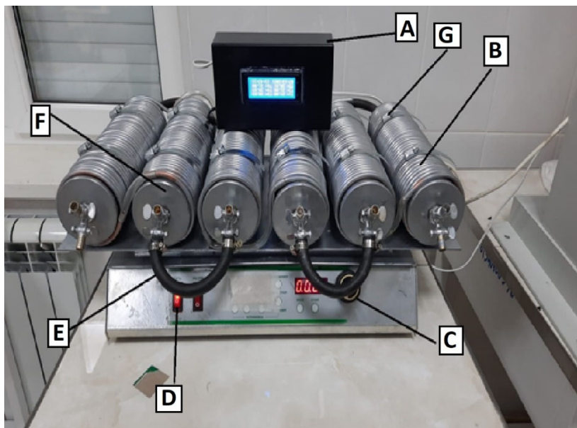
Fig. 4. A multi-stage plug flow reactor for continuous liquid mixing.
