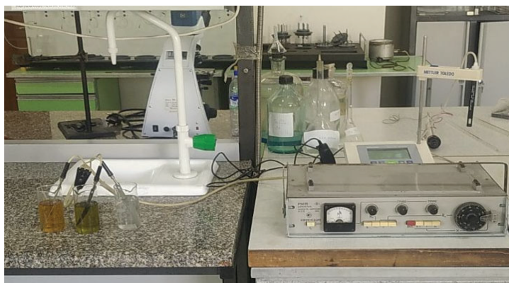
Fig. 2. Device R-5035 for determination of corrosion rate by polarization resistance method.
