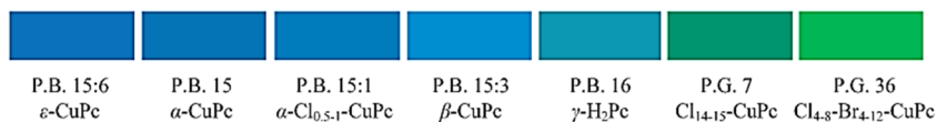
Fig. 1. Shades of the main phthalocyanine pigments based on commercially available pigments from Heliogen (trademark of BASF) [8].
