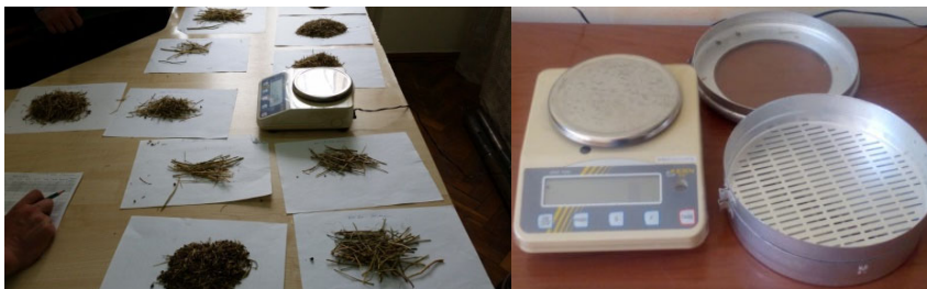
Fig. 2. Tracking the change in the average weighted fraction length of the shredded product from 2 to 20 mm on the screen classifier.
