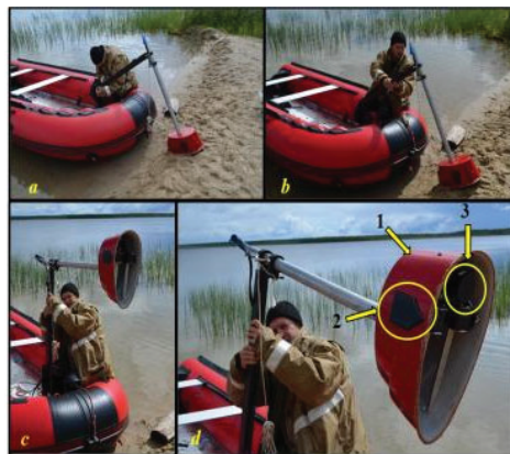
Fig. 2. Installation and location of the fairing (a-c) with hydroacoustic antennas-receivers (d) in the bow of the boat: 1. Fairing body; 2. Antenna-receiver for horizontal echo sounding; 3. Antenna-receiver for vertical echo sounding.
