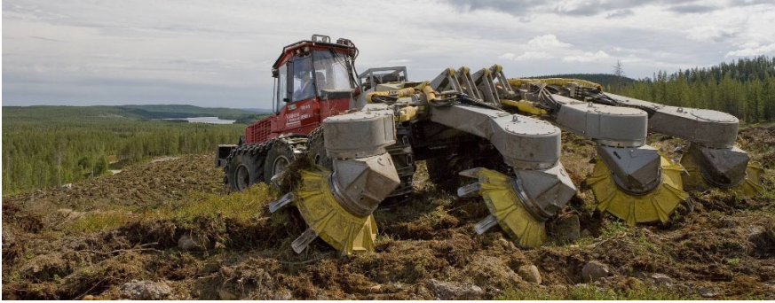
Fig. 3. Milling working body of the Bracke T45 installation.
