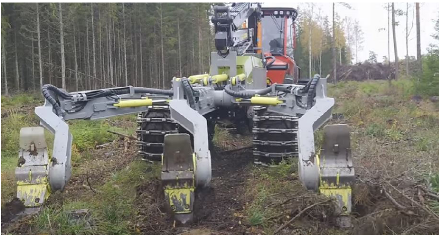
Fig. 4. Discrete working body of the Bracke T26 installation.
