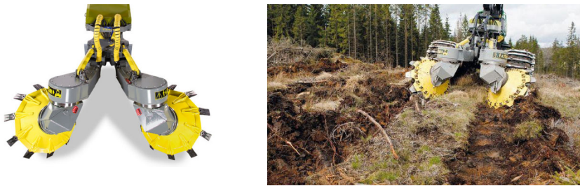
Fig. 2. Milling working body of the Bracke T26 installation and the result of soil milling during reforestation.
