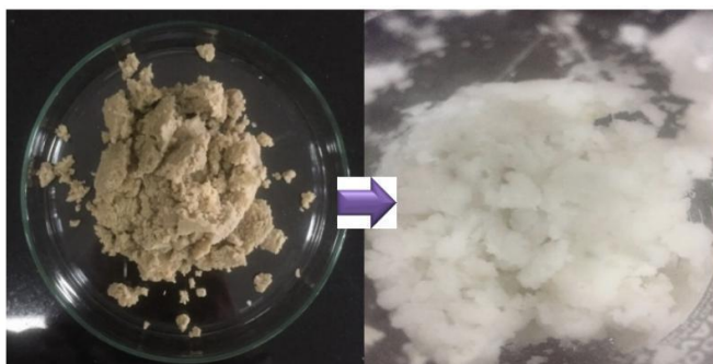
Figure 4. (a) Oil palm trunk powder, (b) Cellulose fibers isolated from oil palm trunk powder. [21]
