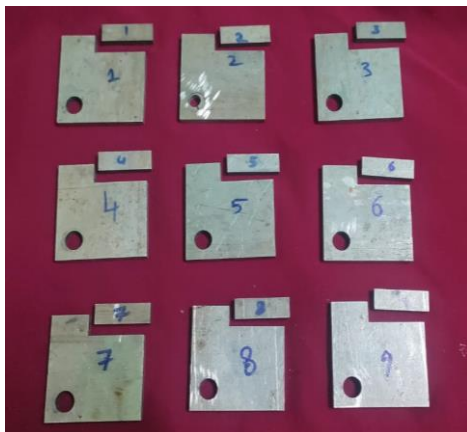
Fig.2. Specimens after cutting with Wire EDM
