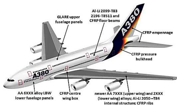
Fig 1. Materials used in Airbus A380 construction [1].
