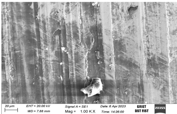
Fig.3. Microstructure of Gas Nitrided Specimen at 12 Hours
