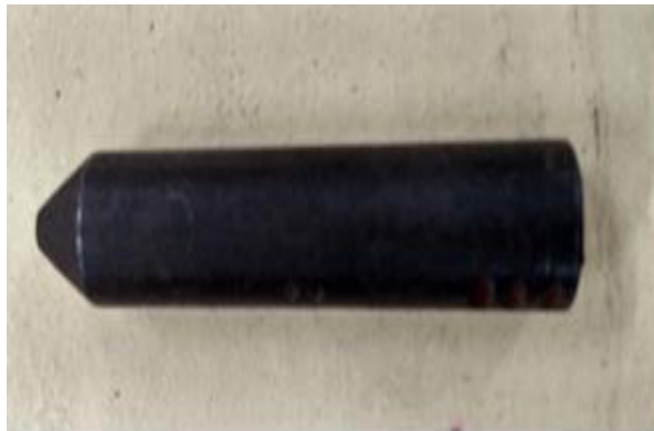
Fig.1. AISI 304 Stainless steel specimen
