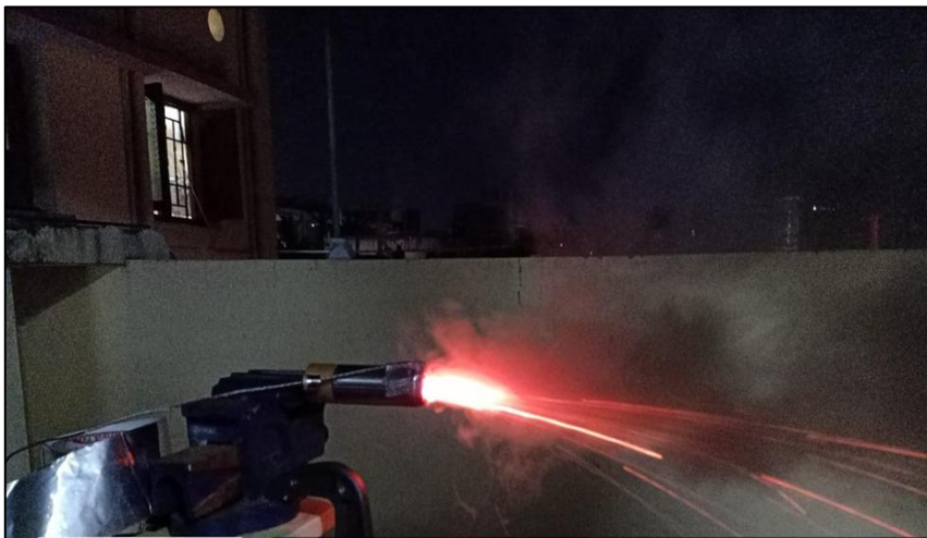
Fig.4 Burning of propellant (Fuel: Lactose, Oxidizer: Potassium Nitrate and Catalyst: Copper)
