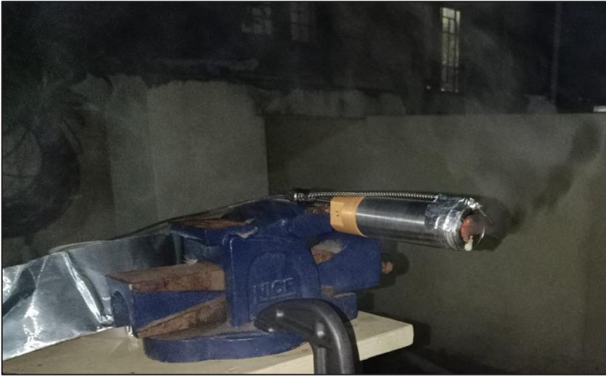
Fig.5 After the burning of propellant (Fuel: Glucose, Oxidizer: Potassium Nitrate and Catalyst: Copper)
