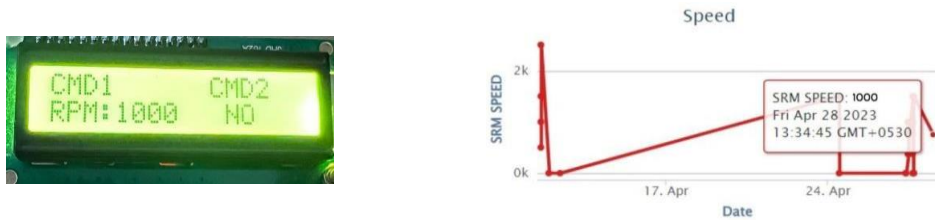
Fig. 12. Display of SRM speed when second CMD1 is given.
