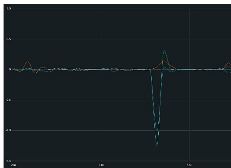
Fig. 5. Graph for 3 axes when the Motorcycle is in the right-side fall maneuver.
