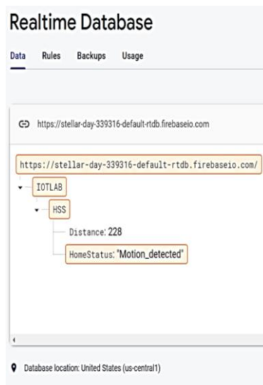
Fig. 8. Realtime firebase when motion detected.
