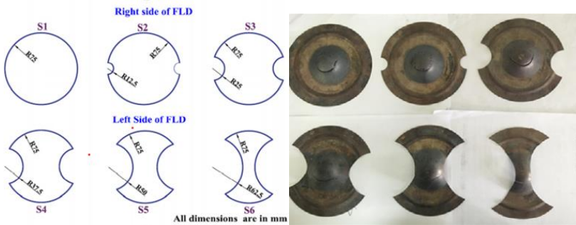
Fig. 7. (a). Specimen geometry studied for the FLDs plots & (b). Stretch formed specimens.
