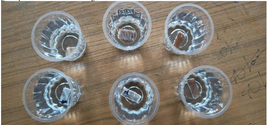
Fig. 7. Specimens meant for water absorption test
