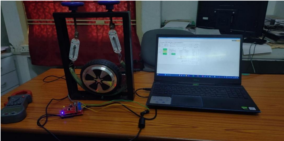
Fig 16. Testing of BLDC Hub Motor
