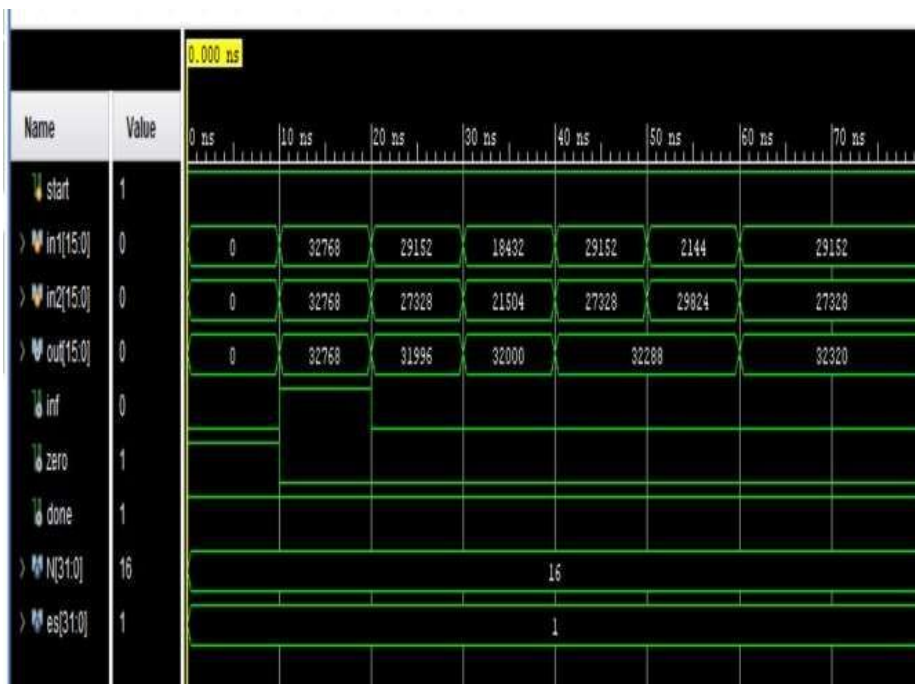
Fig. 5. Simulation results for POSIT MAC Unit
