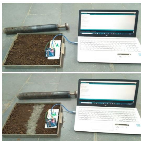
Fig 3. Vibration testing by using fly ash barrier and without using fly ash barrier
