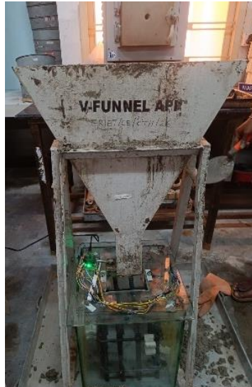
Fig. 3. Test performance while filling the glass column
