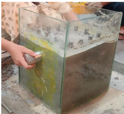
Fig. 5. UPV measurements at 3 sections
