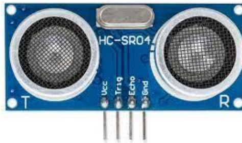
Fig. 1. Ultrasonic sensor (hc-sr04 module)
