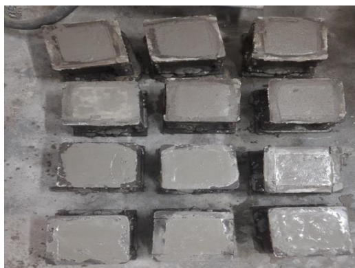
Fig 5 : Casting of Specimens for different Proportions
