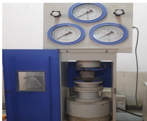
Fig 6 : Experimental Setup for Compression test
