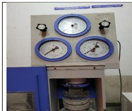
Fig.4 Compressive Testing machine with sample
