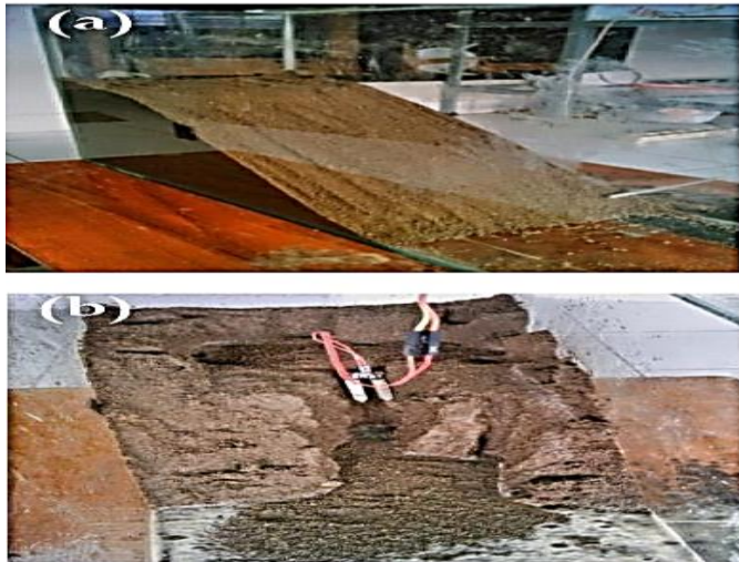
Fig. 5. Landslide simulation before (a) and after (b) the event in soil with sensors
