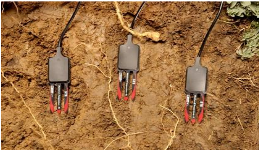
Figure 7. Soil Moisture Sensors
