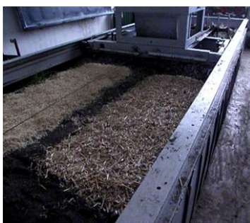
Fig. 3. The preparation of soil channel for conducting experiments on quality of plant residues incorporation.
