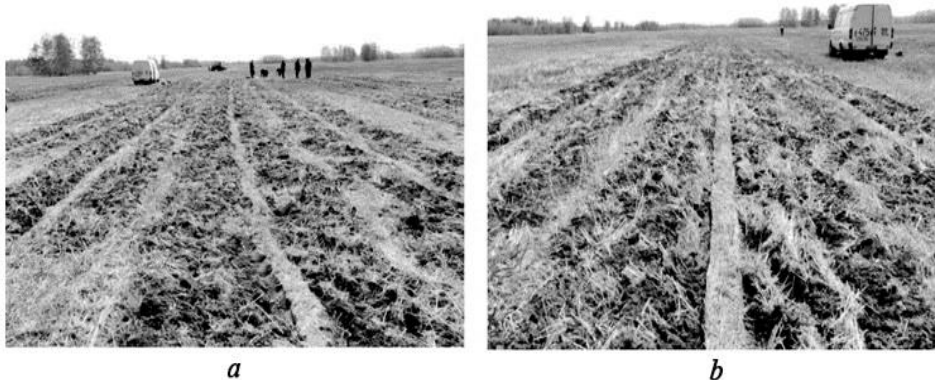
Fig. 7. The height of ridge: a) hexagonal disk; b) round disk.
