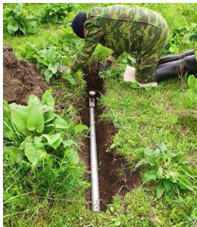
Fig. 2. The survey compass positioning for the MTC-50 device into the trenches (Photo by ©Research station RAS in Bishkek).
