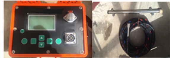
Figure 8. CX806D type foundation pit slope measuring instrument
