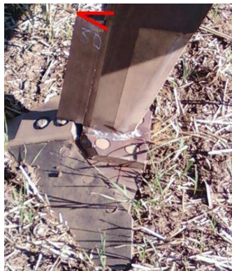
Fig. 2. Sharpening angle of the plane cutter rack
