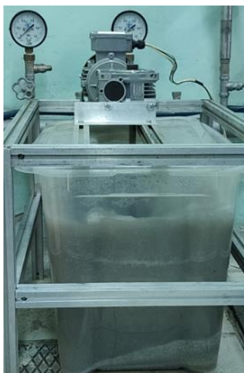
Fig. 3. Experimental bench for testing coatings for resistance to hydroabrasive wear.
