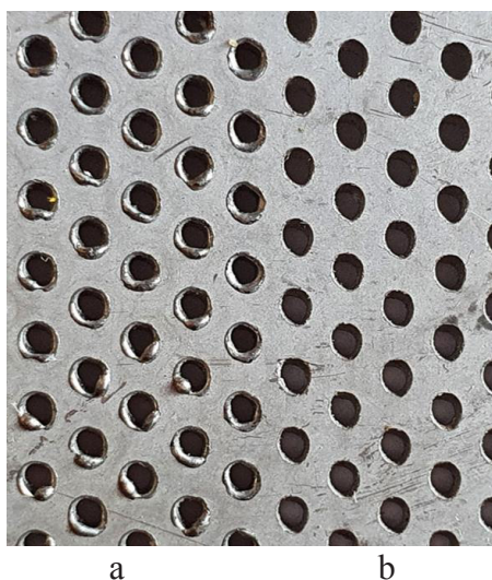
Fig. 2. A fragment of the filter wall from 12H18N10T steel after an electron beam treatment with a thickness of 1.0 mm. The diameter of the hole is 0.6 mm a) from the side of the beam entrance; b) after removal of the burr by chemical-mechanical treatment with metal granules
