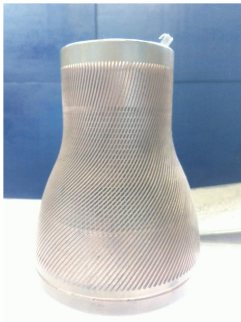
Fig. 1. General view of combustion chamber shell of liquid-propellant rocket engines.
