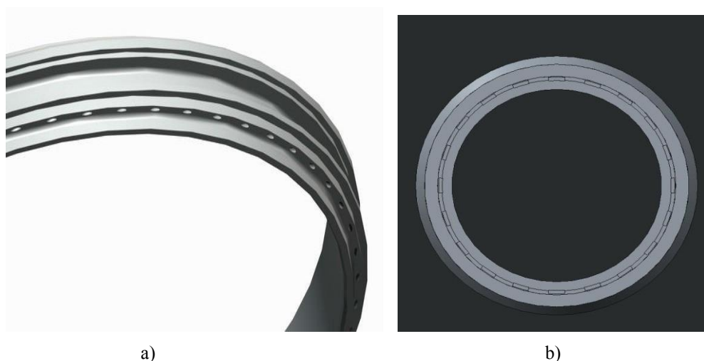
Fig. 2. General view of veil belt of the combustion chamber shell: a) with tangential holes, b) with slot channels.
